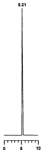
Fig. 4. HPLC chromatogram of purified tracer (gamma counting detection).
